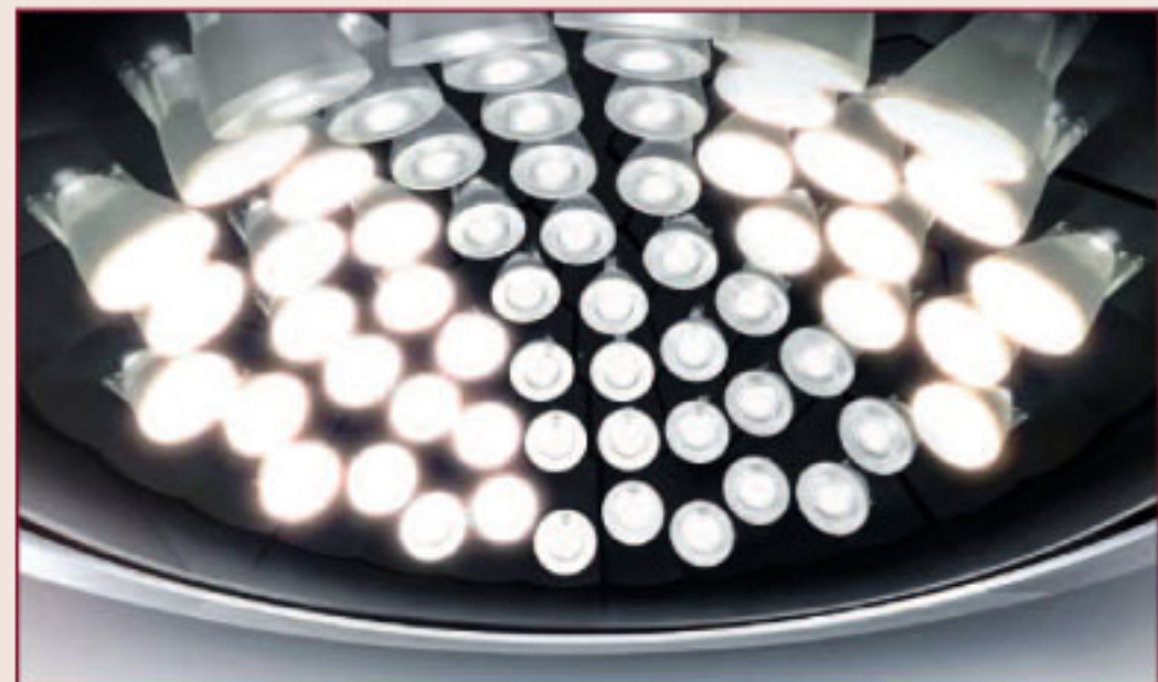
Figure 2: Detail of the "Omnipoint" demonstrator: Each LED with its own lens shines into a different angle and therefore illuminates a different area in the room
