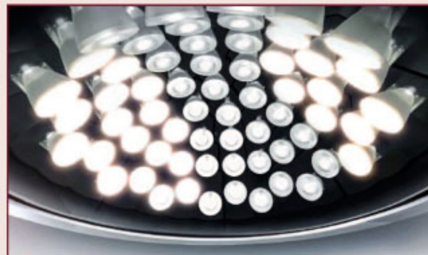
Figure 2: Detail of the "Omnipoint" demonstrator: Each LED with its own lens shines into a different angle and therefore illuminates a different area in the room
